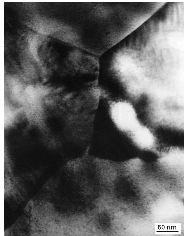
Figure 10 TEM micrograph of a PNN-PZT sample fired at 1125 °C showing a three-grain junction free of liquid phase.
