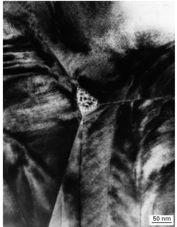
Figure 4 TEM micrograph obtained on a PZT multilayer sample fired at 1125°C, showing a triple point filled with a liquid phase containing phosphorus.
