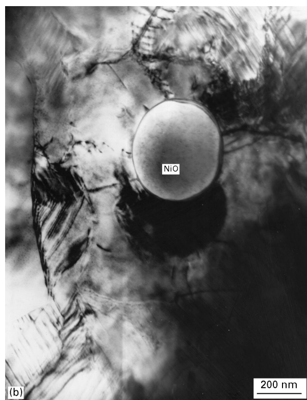
Figure 7 TEM micrograph of PNN–PZT sample sintered at 1125^\circ\text{C} , showing inclusions of (a) \text{ZrO}_2 and (b) \text{NiO} .
